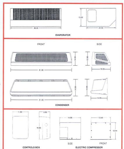
SPECIFICATIONS SUBJECT TO CHANGE WITHOUT NOTICE. Cooling temperature/Capacity ambient 100°F (37.8°C)
